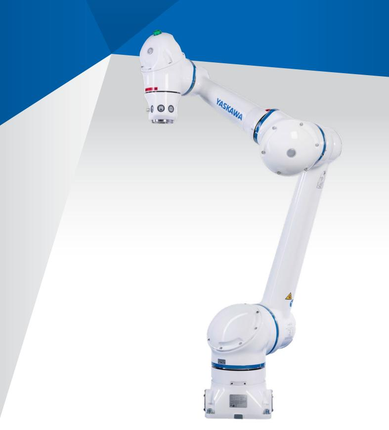
MOTOMAN HC10DT IP67 (B10 + B12) are 6 axes human-collaborative robots with a payload of up to 10 kg. They comply with EN 60529-IP67 and are dust and waterproof for use in harsh environments. Operator safety is ensured by power and force limiters that stop the robot in the event of contact with the operator.
