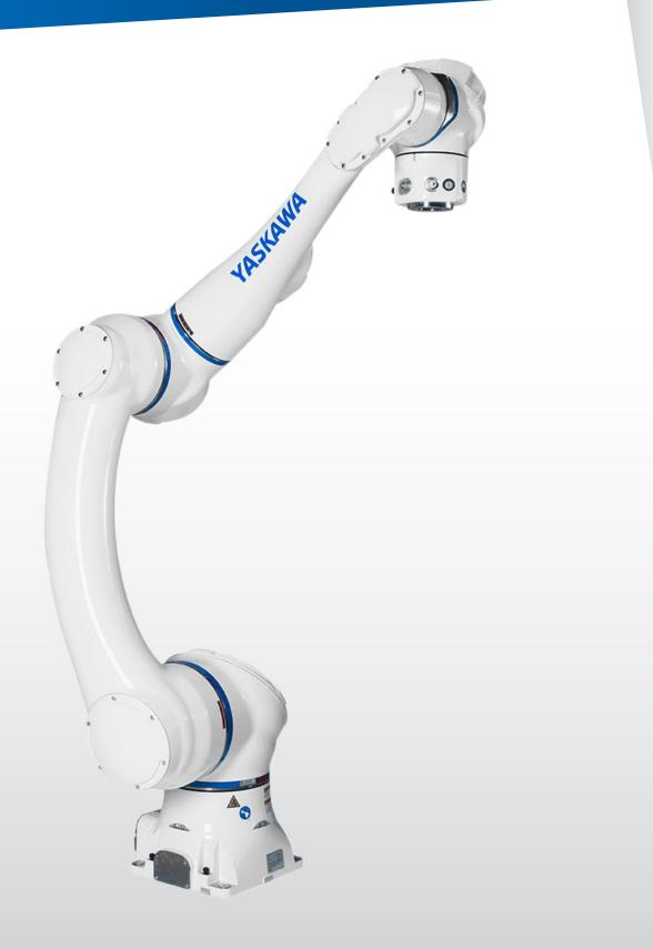
MOTOMAN HC30PL is a 6 axes human-collaborative robot with a payload of up to 30 kg. Operator's safety is assured by a power and force limit technology that stops the robot in case of contact with an operator.
